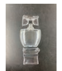
Scrap generated from molding eye drop containers
