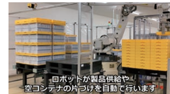
Robots automatically supply products and clean up empty containers.
