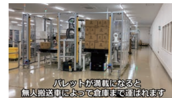
When the pallets become full, they are transported to the warehouse by unmanned vehicles.
